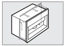
If there is no sealing strip around the installation recess, stick the Miele sealing strip onto the appliance from the back before putting it into the recess. Sealing strips are available from Miele.
